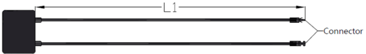
Fig. 13 (1) The full-cell module junction box
