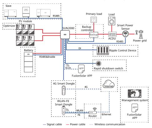
Figure 2-2 Networking application (dashed boxes indicate optional components)
