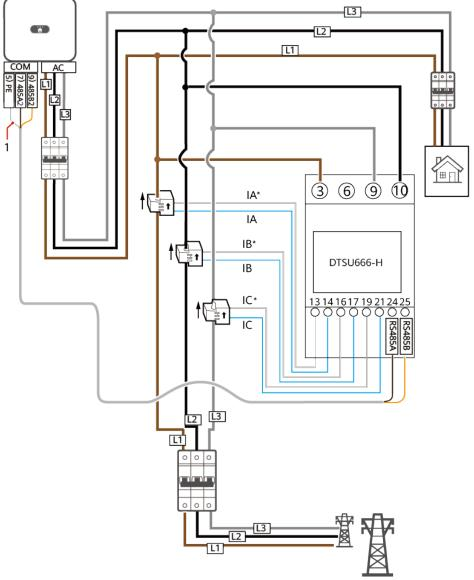
Figure 5-23 Cable connection (Three Phase Three Wire)
