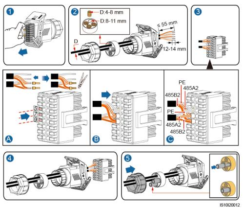
Step 2 Connect the signal cable connector to the COM port.
