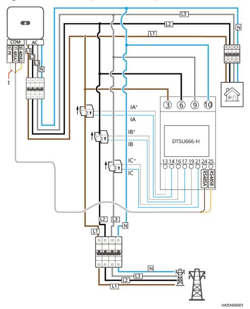
Figure 5-24 Cable connection (Three Phase Four Wire)
