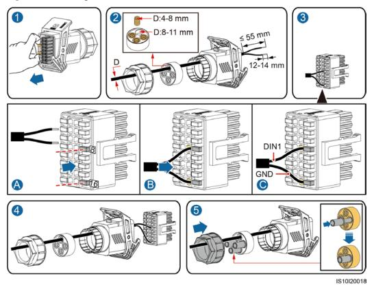
Step 2 Connect the signal cable connector to the COM port.
