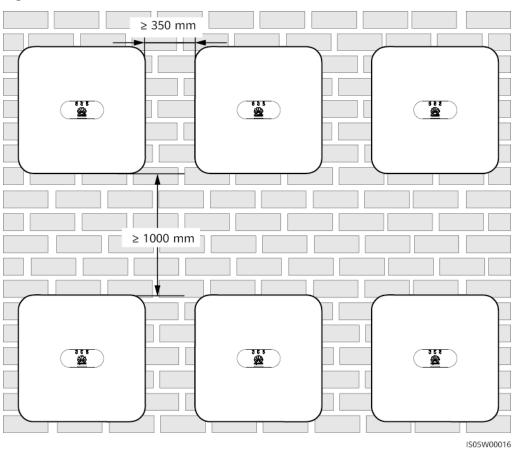
Figure 4-5 Stacked installation (not recommended)
