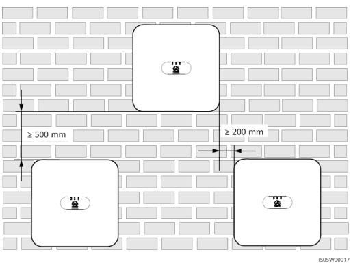
Figure 4-4 Staggered installation (recommended)
