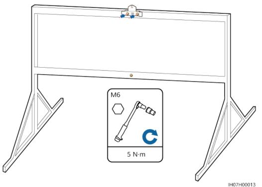
**Step 4** (Optional) Install the locking screw for the DC switch.
